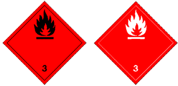
(No. 3) Symbol (flame): black or white; Background: red; Figure "3" in bottom corner
